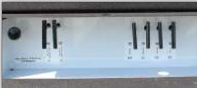
Hydraulic Extend outriggers and over-ride controls are standard on 10,000 lb & larger cranes, and are available as an option on smaller cranes. Manual crank or manual extend are also available for smaller cranes.
