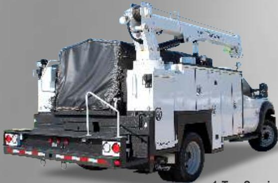
1-Ton Service Body with H6520 Crane & Soft Top Sliding Cover
