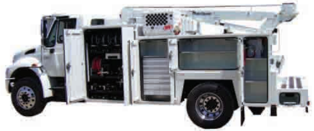
2-Ton Service Combo Body w/8000TT Crane
