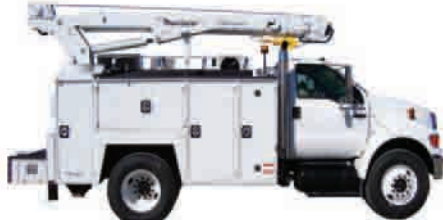
2-Ton Service Body w/10000ST Series Crane (84" CA)
