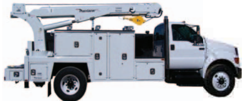
2-Ton Service Body w/12000TT Series Crane with welder platform (120" CA)
