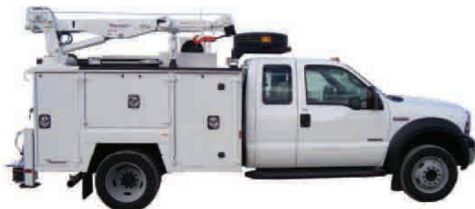
Short tower crane shown
