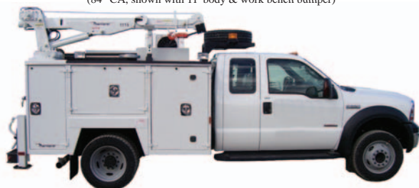
1-Ton Service Body w/1115ST Crane (60" CA, shown with 9' body & step bumper and manual outriggers)
