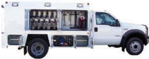
1-Ton Lube Body (side pump & rear reel access)
