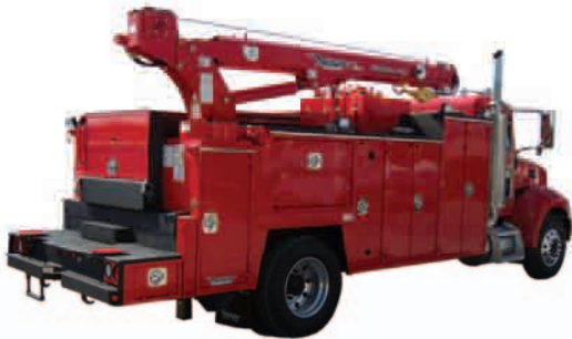
2-Ton Service Combo Body w/8000ST Crane
