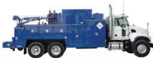
2-Ton Service Combo Body w/1115ST Crane
