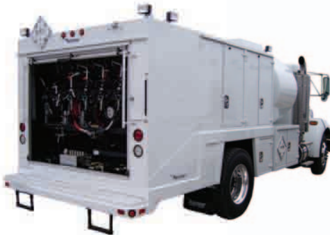
2-Ton Lube Body w/Oval Tank (rear pump & reel access)
