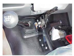
Figure #3 shows a neutral safety bracket in the normal driving position.
