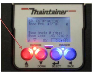
The Status Error Light also show issues. The PWR/COM are used for data transfer and output.
