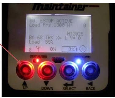
The Status Error Light also show issues. The PWR/COM are used for data transfer and output.
