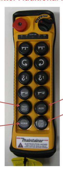
Aux / Air Compressor Engine Start-Engine Stop
