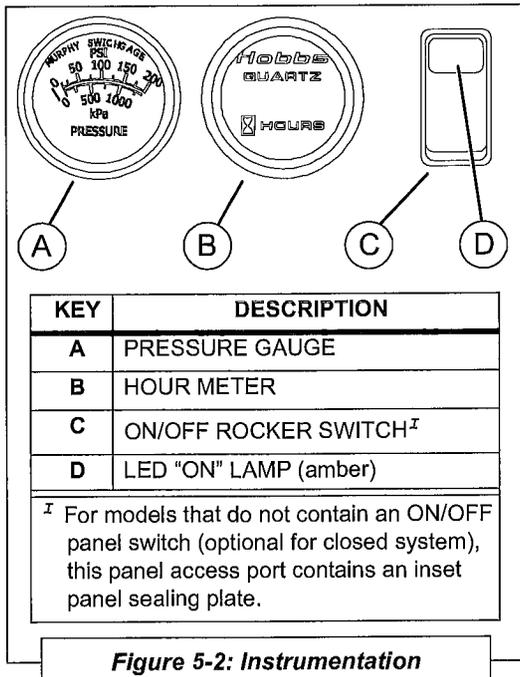
Figure 5-2: Instrumentation
