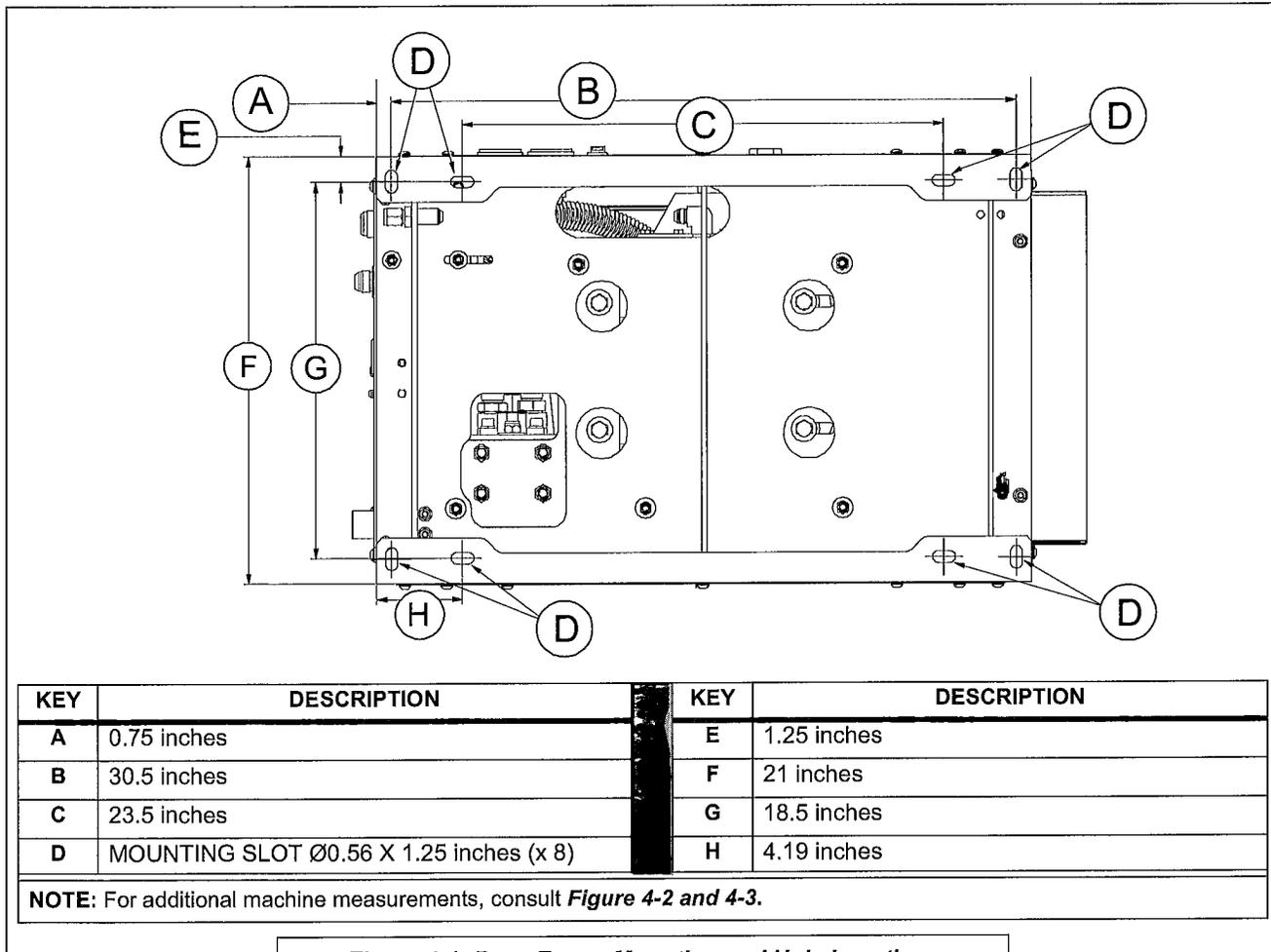
**Figure 4-1: Base Frame Mounting and Hole Locations**
