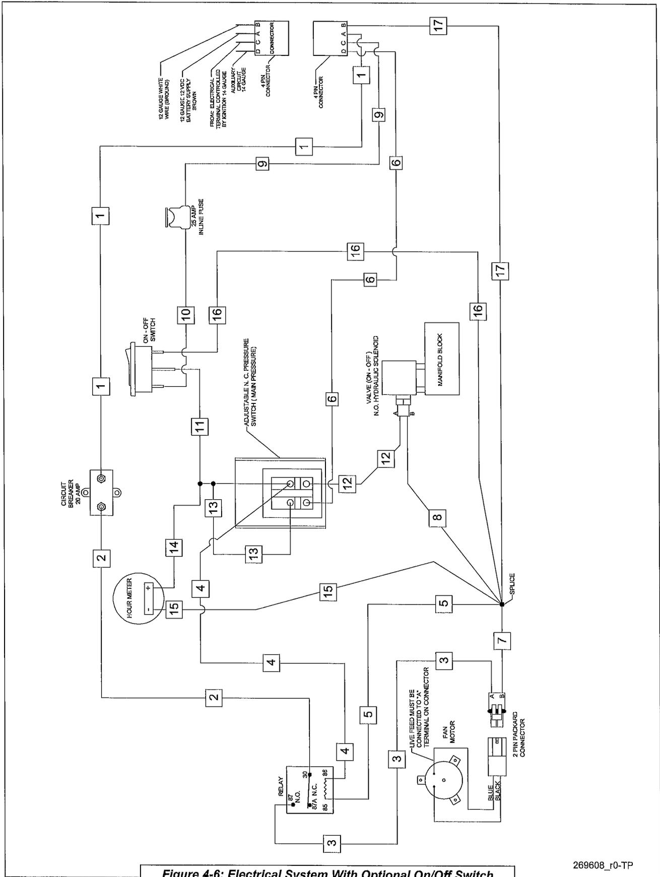
Figure 4-6: Electrical System With Optional On/Off Switch
