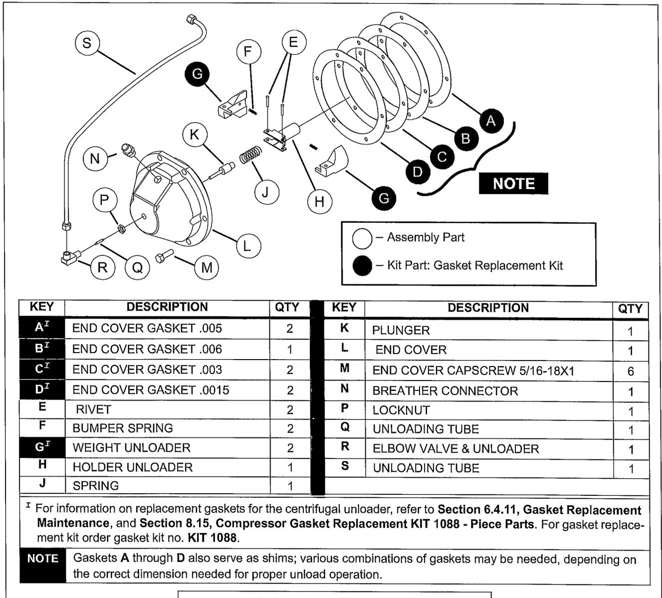
**Figure 6-8: Centrifugal Unloader Maintenance**
