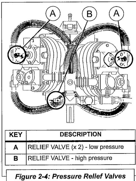
Figure 2-4: Pressure Relief Valves
