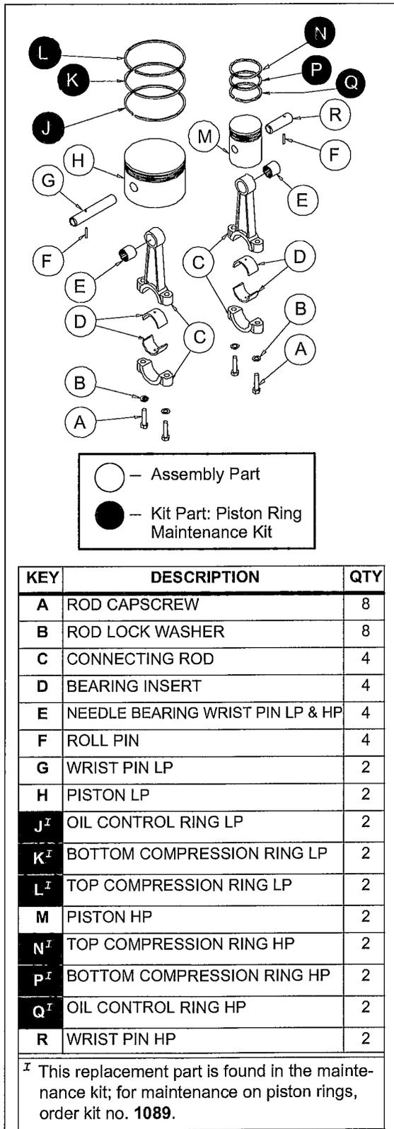
Figure 6-9: Piston Ring Maintenance
