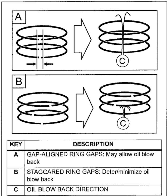
Figure 6-11: Staggered Piston Ring
