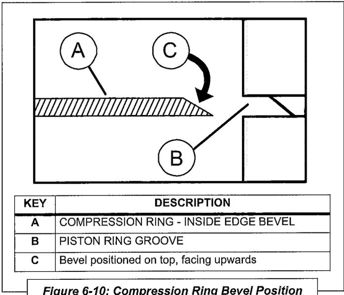
Figure 6-10: Compression Ring Bevel Position
