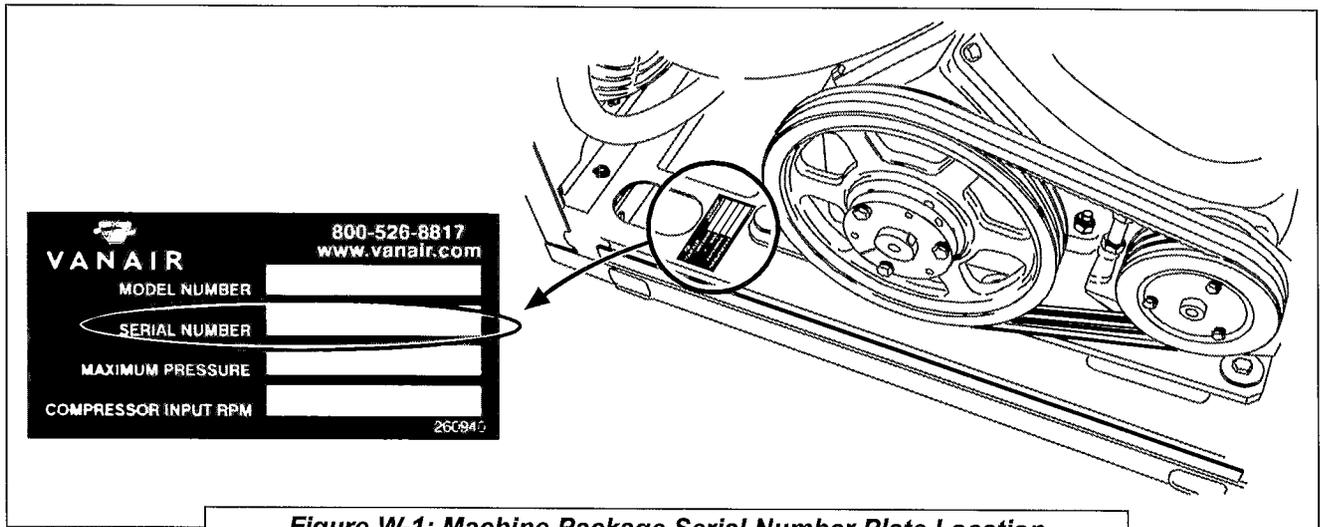
*Figure W-1: Machine Package Serial Number Plate Location*
