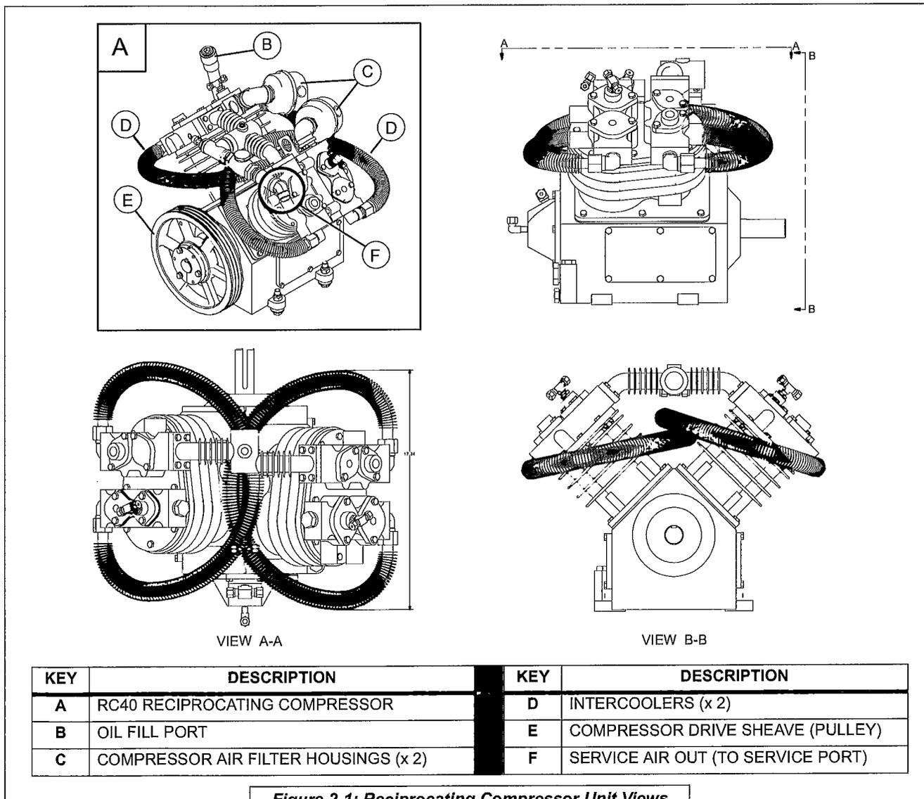
Air is drawn in through dual oversized, dry-type air filters that are located on the compressor pump to provide easy access and long service life.
