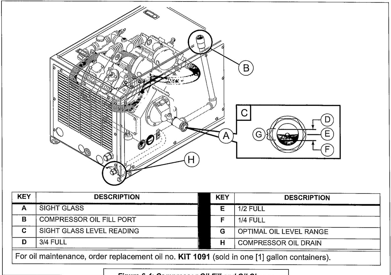
**Figure 6-4: Compressor Oil Fill and Oil Change**
