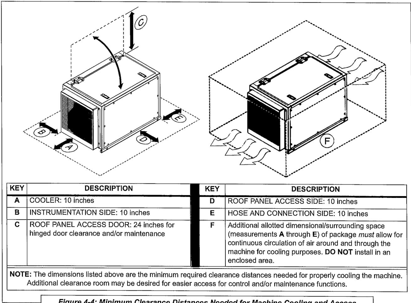
**Figure 4-4: Minimum Clearance Distances Needed for Machine Cooling and Access**
