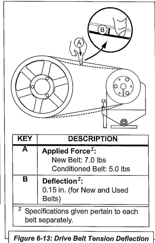
that the compressor pulley always remains stationary during adjustment.
