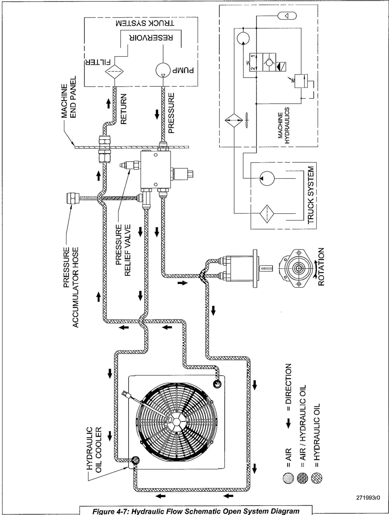
Figure 4-7: Hydraulic Flow Schematic Open System Diagram
