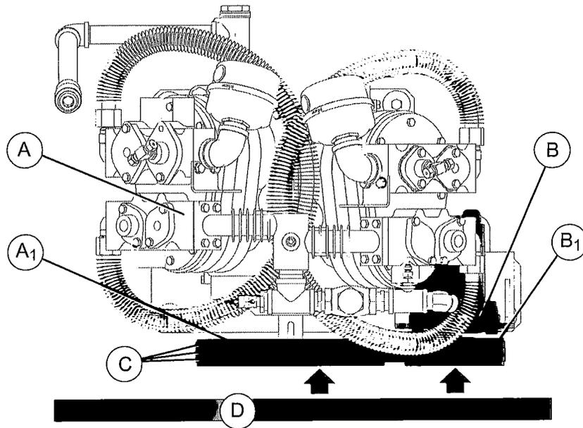
With straight edge flush against both compressor and motor sheaves...
