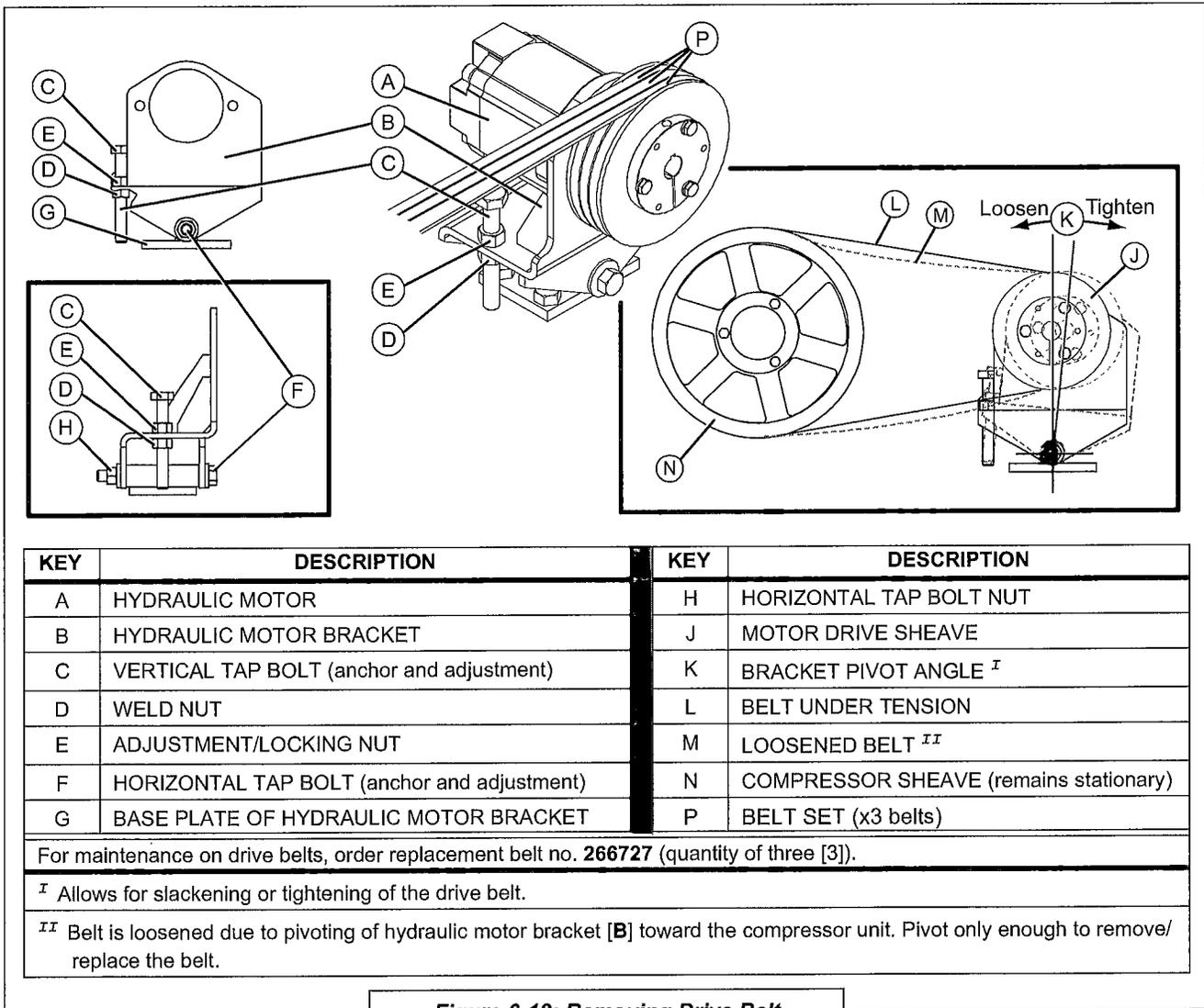
**Figure 6-12: Removing Drive Belt**
