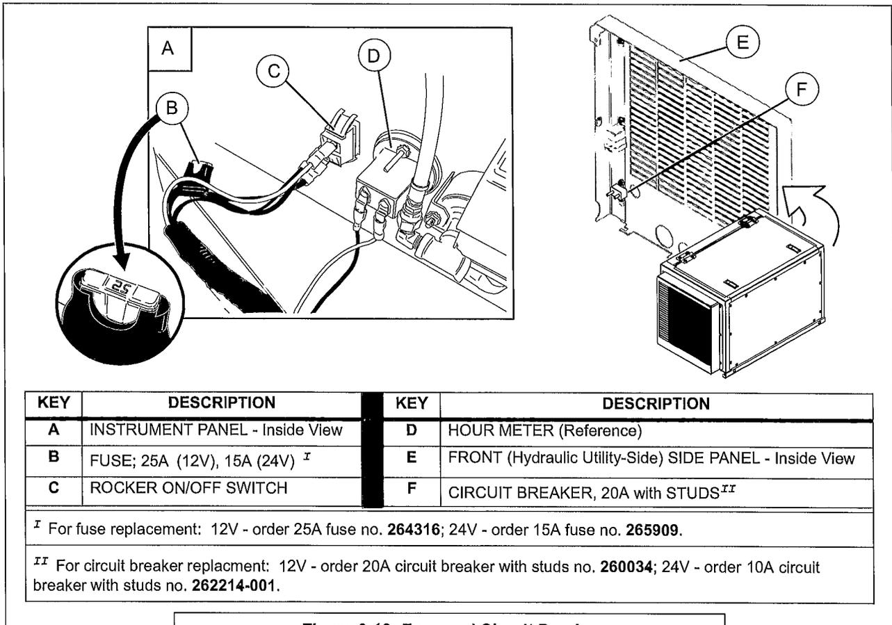
Figure 6-18: Fuse and Circuit Breaker
