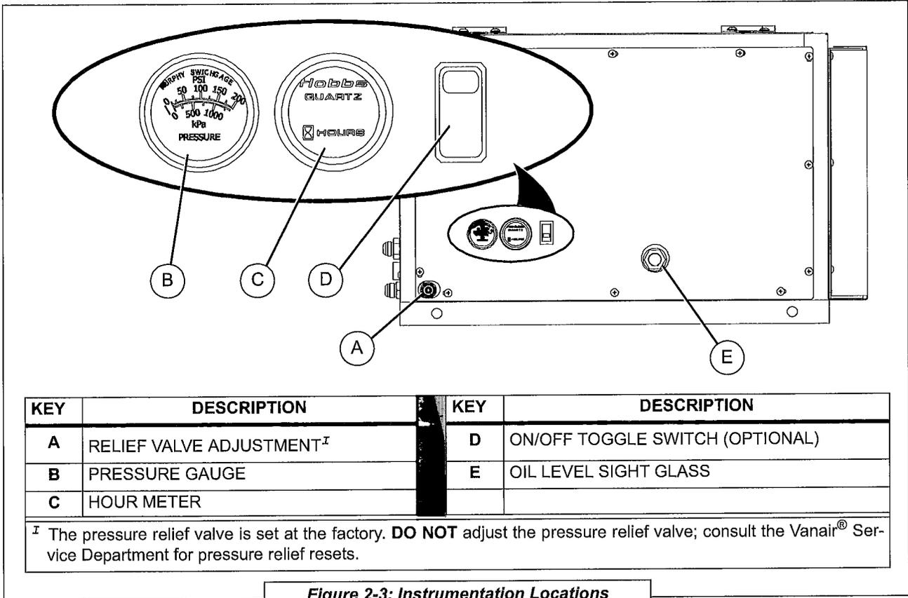
Figure 2-3: Instrumentation Locations
