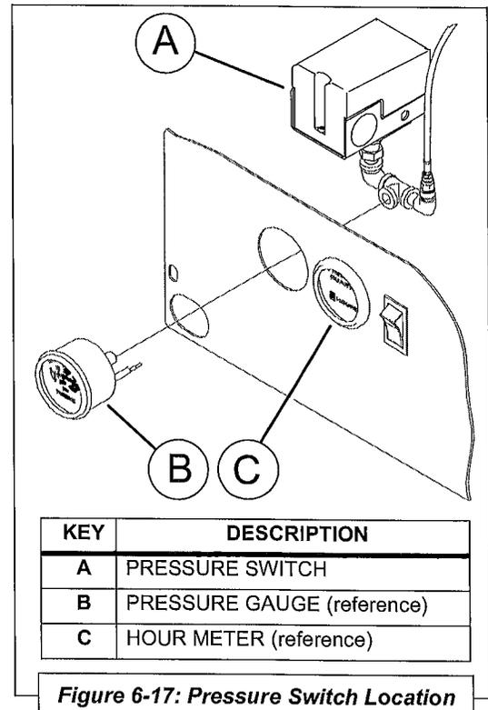
Figure 6-17: Pressure Switch Location
