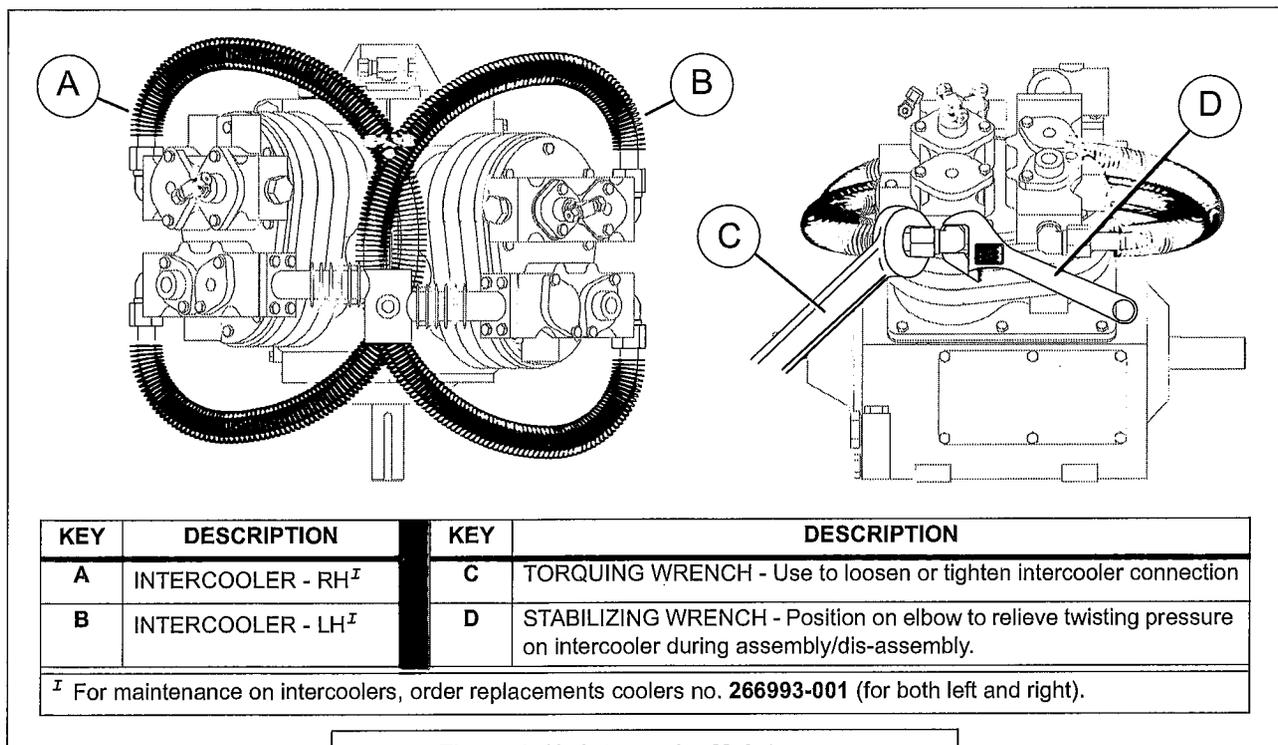
**Figure 6-19: Intercooler Maintenance**
