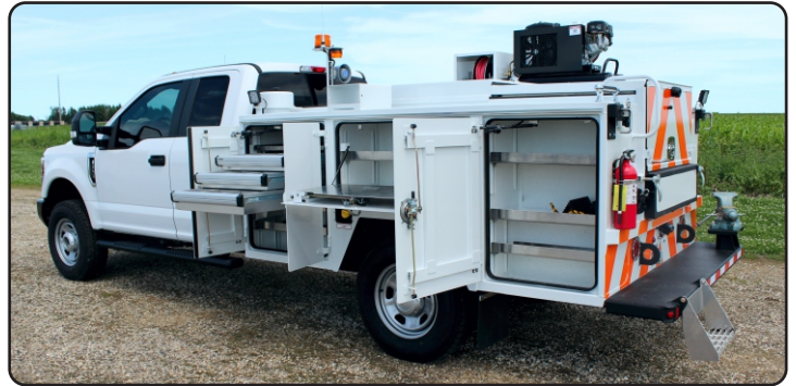
180160 - 9' long aluminum body with 42" high x 16" deep compartments.
