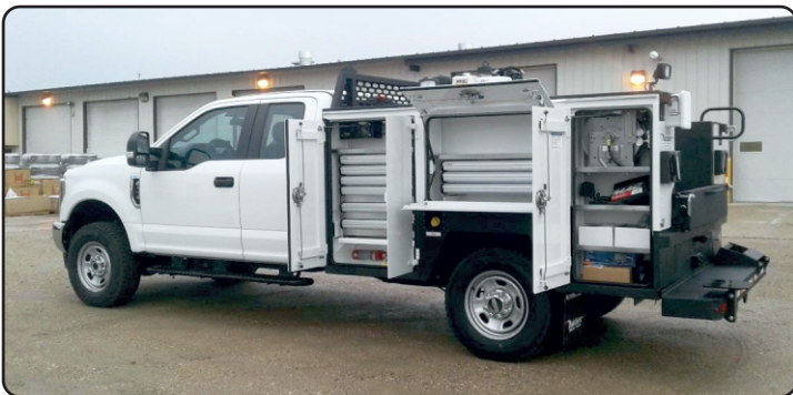
190367 - 9' long aluminum body with 52" high x 16" deep compartments.
