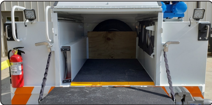
190377- 9' long aluminum body with covered center deck compartment.
