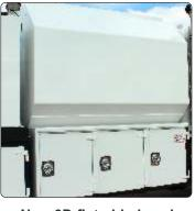
New 8D flat-sided oval diesel tank saves weight the cabinets under 8D tank are all-aluminum
