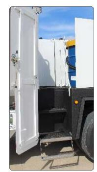
New center deck access wider with illuminated stairway and 3-point contact
