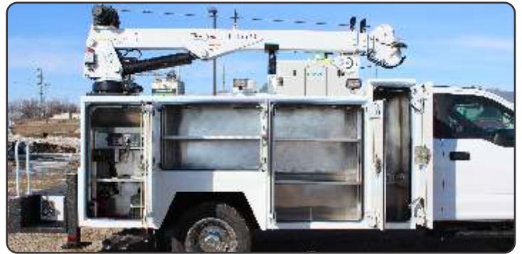
190592 - 11' long aluminum body with EH5520 short tower crane with 5500 lb. max capacity and hyd. extend 10'-20'.
