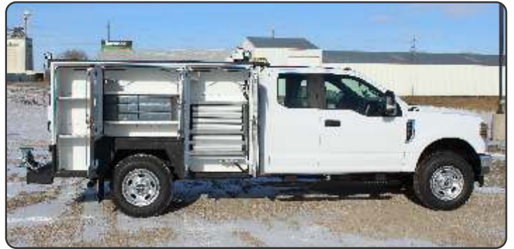
180621 - 9' long aluminum body with 60" high x 16" deep compartments.
