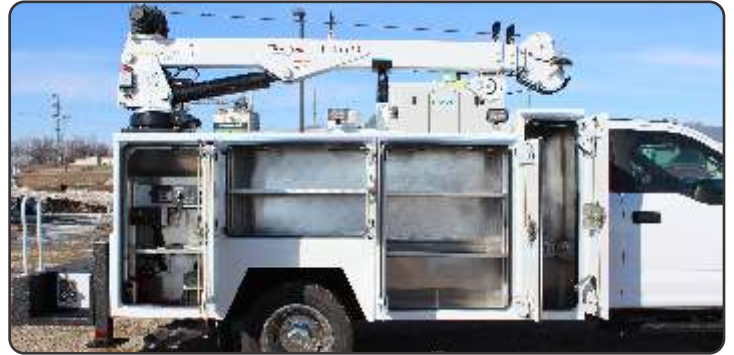
190592 - 11' long aluminum body with EH5520 short tower crane with 5500 lb. max capacity and hyd. extend 10'-20'.
