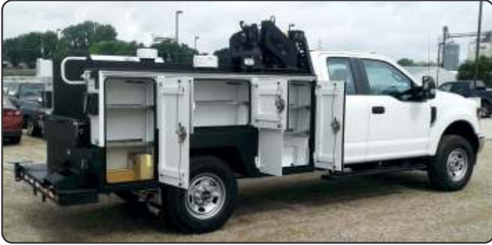
190297 - 9' long aluminum body with 52" high x 16" deep compartments.
