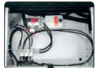
12vDC Power Pack for Hydraulic Outriggers
